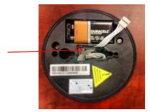
• Be careful not to crimp or damage the lock cable upon EntryPad installation.
