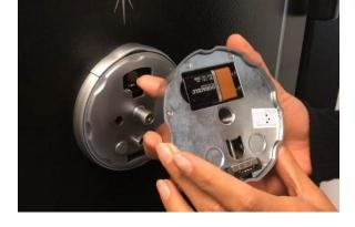
Step 6: Pull down the Spin Dial release and try your electronic codes to open the safe door.
