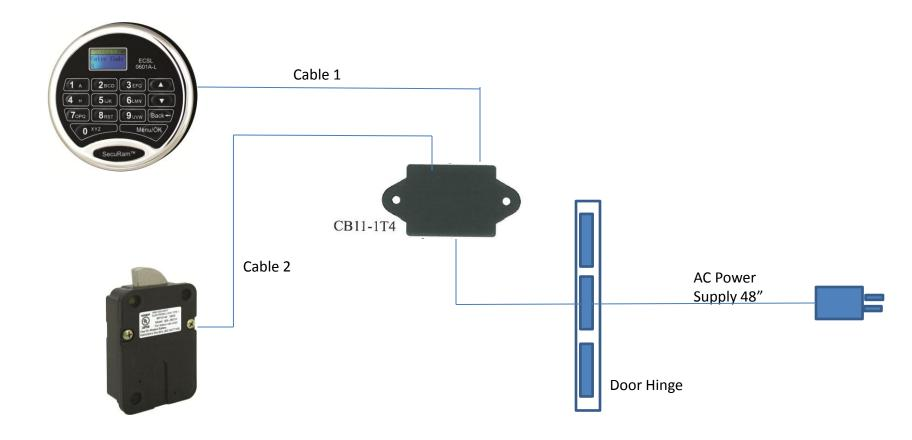
Here is a standard AC Power wiring diagram
