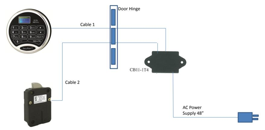
Here is an alternate AC Power wiring diagram, where the Junction Box is inside the safe
