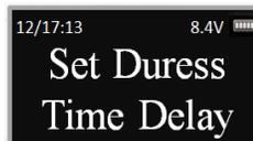
Step 5: Press the  $\uparrow$  and  $\downarrow$  to adjust the Time Delay value (0-99 minutes). Press OK.
