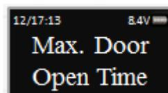
Step 5: You will be prompted to enter the maximum length of time the door can be opened., after which the LCD will report an alert indicating that the door opening has exceeded the allowable time limit,- the lock sound with an audible beep.
