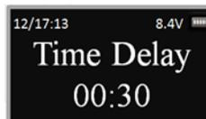
Step 4: When Time Delay expires, the entrypad will beep twice then display: "Time Window XX:00", indicating the length of time the User has to enter a valid user code to gain entry.
