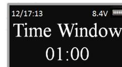
The Counter will count down until the Time Window has expired. A user code is used to open the lock.
