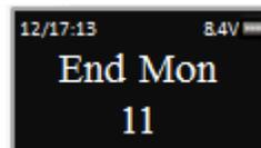
Step 10: (*Ending Week*) The system will now request the Week in which Daylight Savings Time is to end. The default is North American DST Week 1 – note – the system calculates this as the 1<sup>st</sup> full week in this month. To change Press the  $\uparrow$  and  $\downarrow$  to set the Week; and press OK
