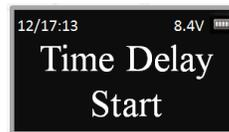
Step 3: Display will flash on every 15 seconds, reaches the preprogrammed time delay value.
