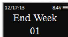
Step 11: (*Ending Time*) The system will now request the Time on the first day of the week (Sunday) at which Daylight Savings Time is to end. The default is North American DST Time 2 – 2:00am. To change Press the  $\uparrow$  and  $\downarrow$  to set the Week; and press OK
