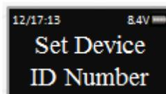
Step 5: Using the numbers on the EntryPad, specify the desired Device ID number for this EntryPad using a four digit number format from 0010-9999 and press OK.
