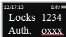
Step 8: In order to authorize access to these individual locks, press the corresponding number on the EntryPad to toggle “O” or “X”.
